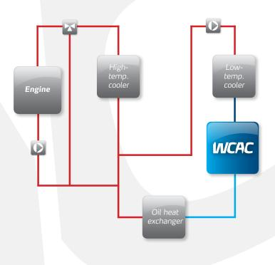
In addition, the WCAC system from Nissens is designed to comply with the applicable emission standards (Euro 6/Tier 4F), since a constant, lower charge air temperature leads to **lower emission levels**. This offers a vital contribution to ensuring environmental benefits and an increasing green focus in the market.
